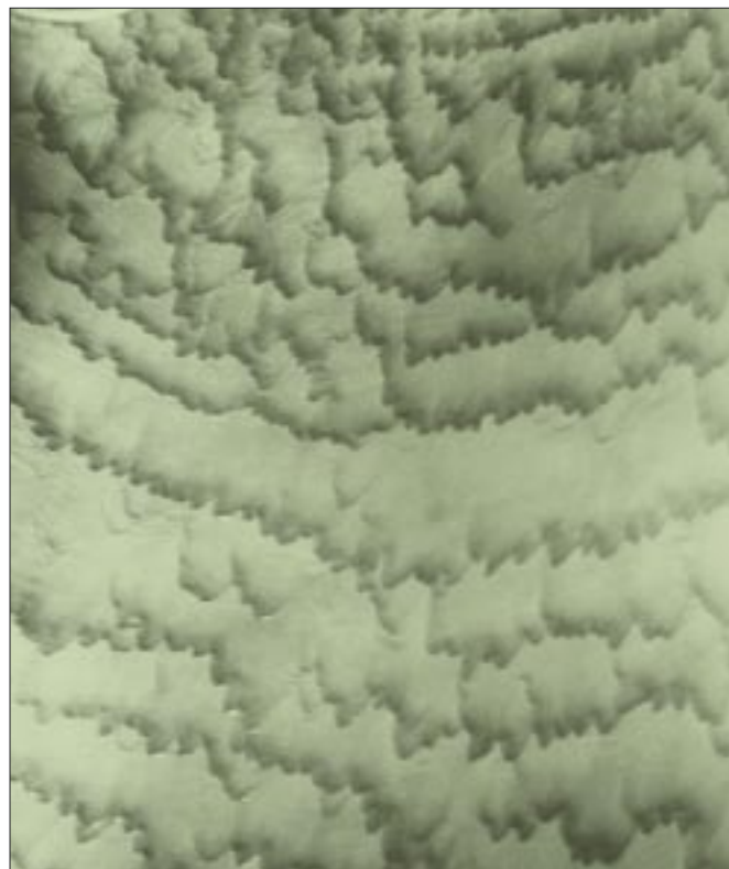
High speed photo of the liquid film on the heat transfer surface of the Centritherm. The film is only 0.1 mm thick and crosses the surface in about 1 second resulting in a well defined residence time. The photo also shows substantial agitation in the liquid film, one of the factors that contribute to the Centritherm's high efficiency.
